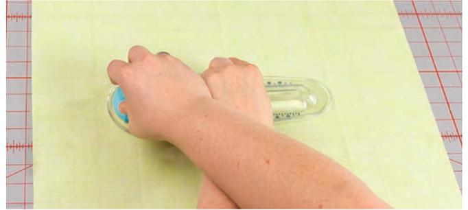
3. Apply pressure to the blade and sizing knobs, and in one smooth motion, rotate the blade knob in a full circle.
