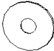
2 - Fender Washers (Largest Size) 1 - 1/2" O.D. 3/8" I.D.
